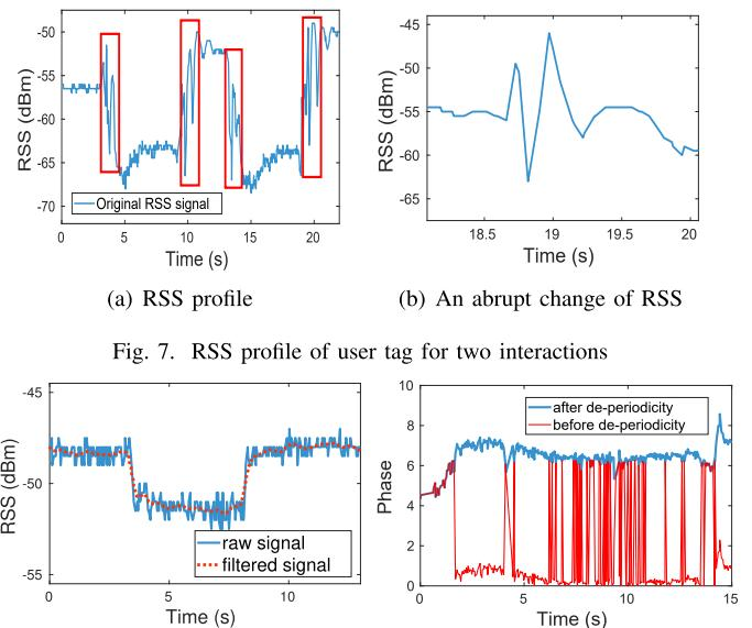
$R_h$  to detect interaction events: if the RSS difference between current and following signal points is larger than  $R_h$ , then the timestamp of this signal point is considered as potential starting/finishing time for tag interaction.
