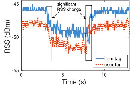
Fig. 4. Signal strength change of two coupling tags
