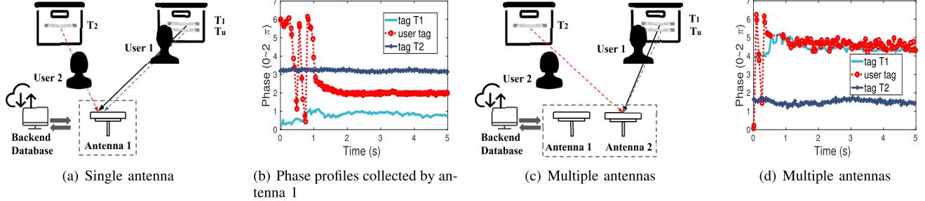
Fig. 5. Phase profiles and differences captured by multiple antennas
